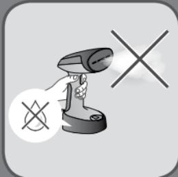
**EN** Allow the appliance to run until the water tank is completely emptied.
