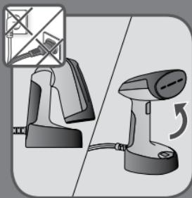
**EN** Always unfold the steam head until it is locked before any use of the appliance.
