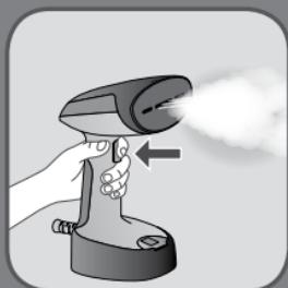
**EN** When the light is steady, release steam by pressing continuously on the steam button away from any garments.
